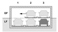
To remove the vehicle from the space in **grid 3/LF**, the GF platforms are moved to the left.
